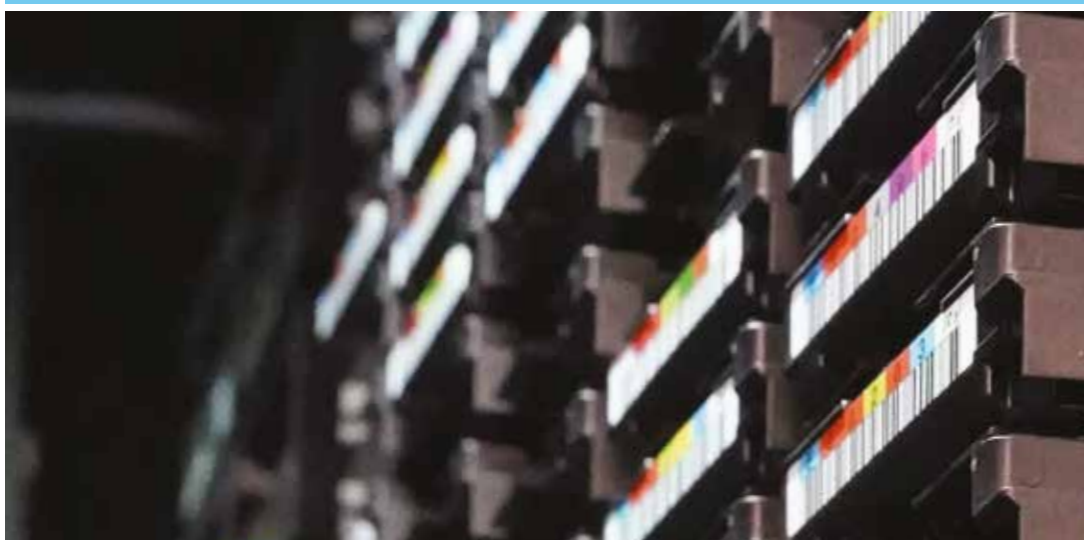
ESI data archive: the tape library is the digital custodian that holds the collected history of every experiment, recording, and analysis performed at the institute safeguarded on magnetic tapes.
