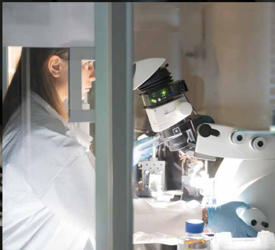
Cutting device (ultramicrotome) allowing us to prepare brain slices as thin as 35 nm (more than a thousand times thinner than a human hair).
