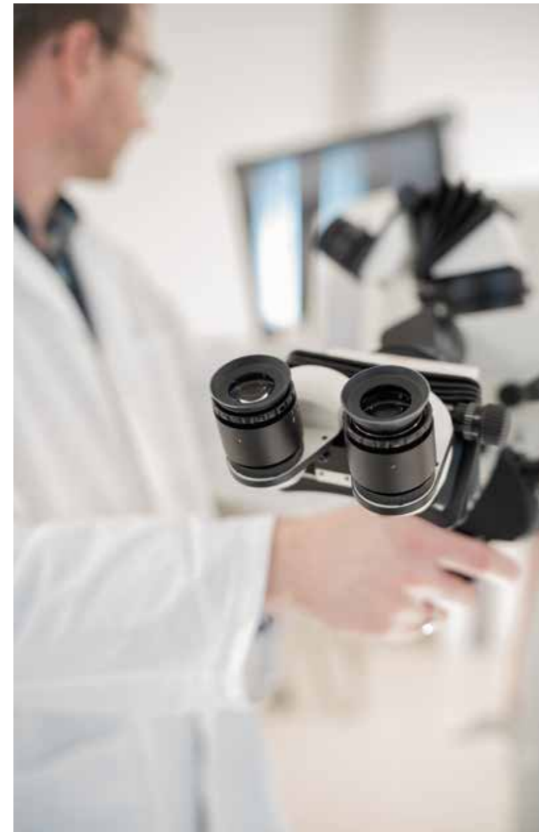
A surgical microscope which, in addition to the classic optics, also contains a camera with which the whole team can follow the surgery
