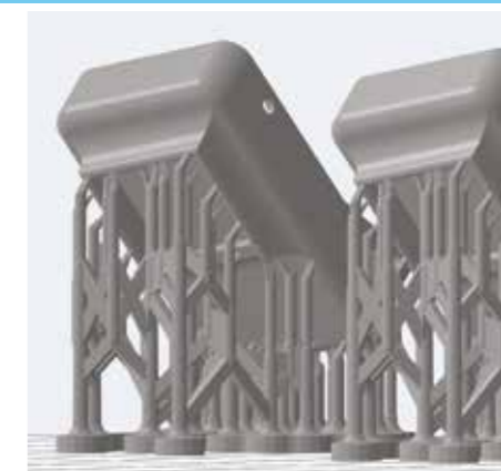
Preparation for a 3D printjob on a stereolithography (SLA) 3D printer. A slicing software uses automatic algorithms to set up the layout of a 3D print - in this case some lids to cover chambers.
